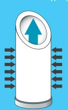
This superfine filter is designed to mechanically remove sediment particles. Grit, dust, rust, mud, algae – all of these are removed in this first stage of filtration.
